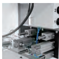
Pneumatic abrasive belt tensioning
