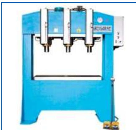
FDM-80/3 E equipped with three independent headstocks.
