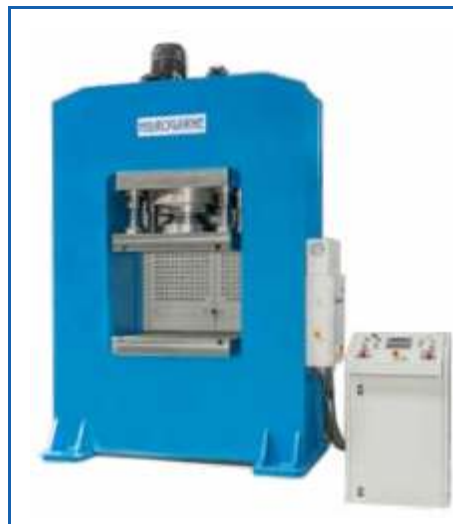
Model RM-500 E with CNC and hydraulic ejector.
