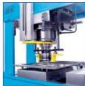
Punching tools set for diameters from 6 to 160 mm.
